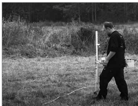
Figure 4. Glenn Envall, Skandinavisk Arkeologisk Geofysik AB (SAGA), conducting a survey with a magnetometer. Photo Staffan von Arbin, Bohusläns museum.
